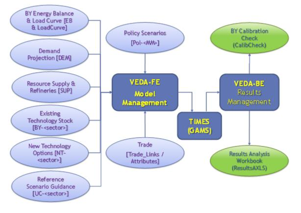
Figure 100: TIMES-CR Model Structure Overview
