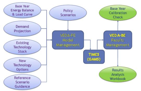
Figure 83: TIMES-Vietnam Modeling Platform Overall Structure
