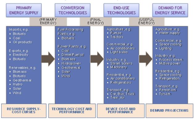
Figure 82: TIMES Basic Components
